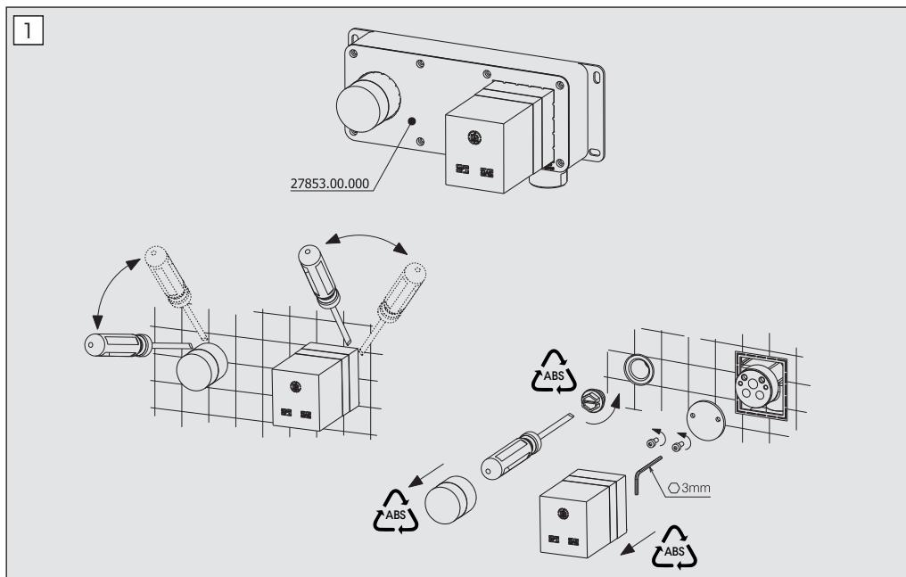
**FASE 1\_PHASE 1\_ÉTAPE 1\_SCHRITT 1\_FASE 1\_1  TAP 1\_FAS 1 步骤— 1 المراحلة 1****IT Fissaggio e connessione miscelatore.**
