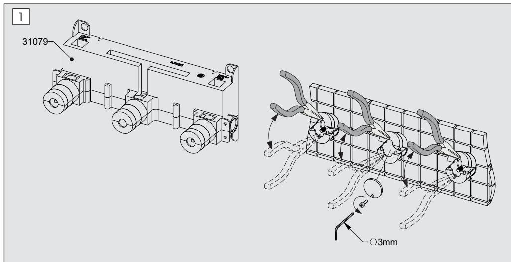
**FASE 1\_PHASE 1\_ÉTAPE 1\_SCHRITT 1\_FASE 1\_1 ЭТАП\_FAS 1 步骤一\_المرحلة 1****IT Fissaggio e connessione miscelatore.**
