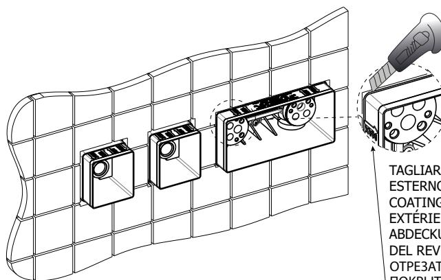
TAGLIARE A FILO DEL RIVESTIMENTO ESTERNO\_CUT FLUSH WITH OUTER COATING\_COUPER À FIL DU REVÊTEMENT EXTÉRIEUR\_BÜNDIG MIT DER ÄUSSEREN ABDECKUNG SCHNEIDEN\_CORTAR AL RAS DEL REVESTIMIENTO EXTERNO ОТРЕЗАТЬ ЗАПОДЛИЦО С НАРУЖНЫМ ПОКРЫТИЕМ\_SKÄR AV JÄMS MED BEKLÄDNADEN\_将覆材切成长条
