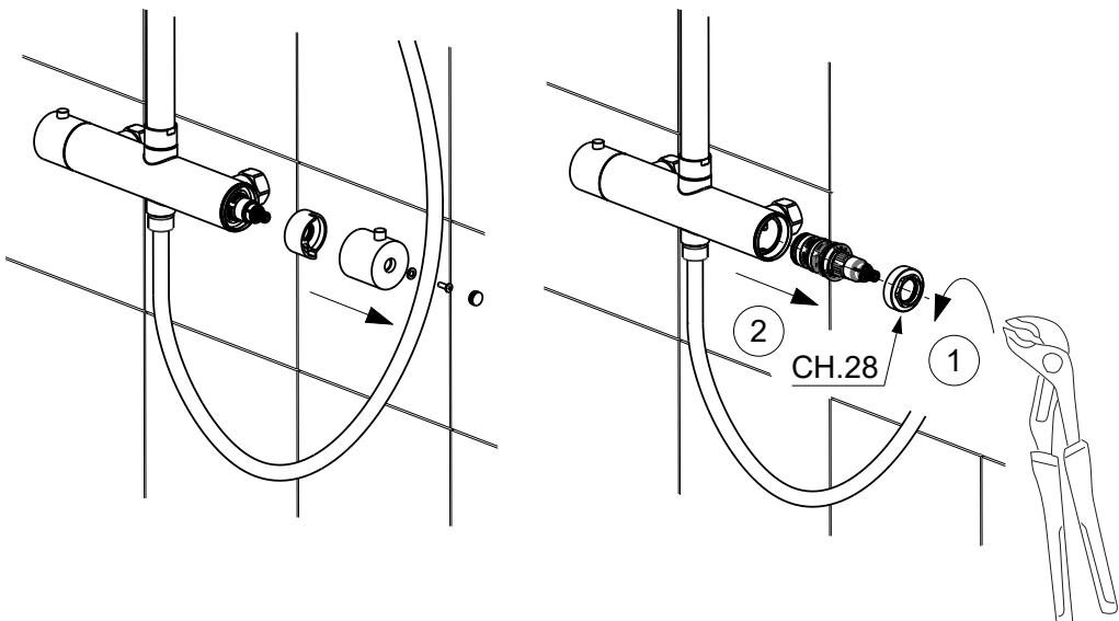
SOSTITUZIONE DEVIATORE\_ DIVERTER REPLACEMENT\_ REMplacement DU COMMUTATEUR\_ DIVERTER ERSETZEN\_ REEMPLAZO DESVIADOR\_ ЗАМЕНА ДИВЕРТОРА\_ BYTE AV AVLEDARPATRON\_ 更换分流器滤芯\_
