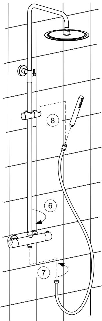
SOSTITUZIONE CARTUCCIA THERMOSTATICA\_ THERMOSTATIC CARTRIDGE REPLACEMENT\_ REMplacement DE LA CARTOUCHE THERMOSTATIQUE\_ THERMOSTATISCHER KARTUSCHENWECHSEL\_ REEMPLAZO DE CARTUCHO TERmostÁTICO\_ ЗАМЕНА ТЕРМОСТАТИЧЕСКОГО СМЕСИТЕЛЯ\_ BYTE AV TERmostatPATRON\_ 更换恒温阀滤芯\_
