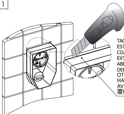
TAGLIARE A FILO DEL RIVESTIMENTO ESTERNO\_ CUT FLUSH WITH OUTER COATING\_ COUPER À FIL DU REVÊTEMENT EXTÉRIEUR\_ BÜNDIG MIT DER ÄUSSEREN ABDECKUNG SCHNEIDEN\_ CORTAR AL RAS DEL REVESTIMIENTO EXTERNO\_ ОТРЕЗАТЬ ЗАПОДЛЦО С НАРУЖНЫМ ПОКРЫТИЕМ\_ SKÄR AV JÄMS MED BEKLÄDNINGEN\_ 将覆材切成长条\_ القطع بقص التكسية\_
